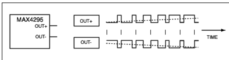
Figure 1. These complementary PWM outputs are generated by a class D amplifier in the bridge configuration (like the MAX4295). The average values of these waveforms (the dashed lines) are produced by an output filter, whose loss and distortion-producing artifacts should be held to a minimum.
